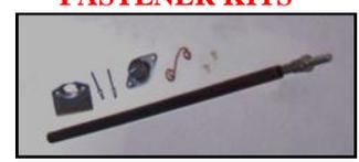
These stands allow Dzusing through the top of the scoop for stable, easy mounting. Each kit contains 12" moly tubing, 1 threaded stud, jam nut, 1 Dzus receptacle, 1 Dzus fastener & spring assembly and instructions.
