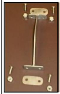
These components are designed to allow the scoop to take severe pressure without opening deflection or allowing the scoop/air pan to separate from the carbs, as it is very important to keep the air box sealed to the carbs.
