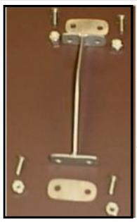
These components are designed to allow the scoope to take severe pressure without opening deflection or allowing the scoope/air pan to separate from the carbs, as it is very important to keep the air box sealed to the carbs.
